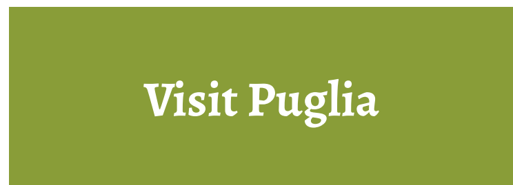
Fig. 2: Suggested combination of white text on green (#839E52). This meets the minimum WCAG contrast ratio of 3:1 for large text.
